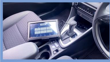
On all models the touch-screen user interface is mounted in a specially designed holster in the front of the vehicle where it can be safely stored when not in use. When in use it can sit on the operators lap for easy operation. TES been at the forefront of mobile CCTV installations since 2004, all systems are built and installed by the TES engineering team in their own dedicated workshop facilities.
